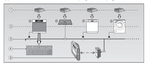
These instructions are for a communication enabled oven ② that can be linked into the Miele@home system via a communication module ① (optional accessory).
